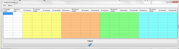
10 different transmitters are possible; each transmitter is made of 4 multiplexes. The menu of this page and the popup menu (right click) are similar to those from the main page. Enter the transmitter name
