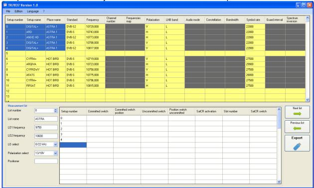
In the case of a simple installation with a single satellite dish, there is no other parameter to enter. Click on the Next list button to create a HOT BIRD measurement list
