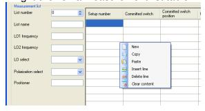
**New** allows you to initialize the setups of the measurement list only. **Copy** allows you to copy in the clipboard the data selected with the mouse. **Paste** allows you to paste the content of the clipboard to the place of the cursor. **Insert line** allows you to insert an empty line in the list above the cursor.
