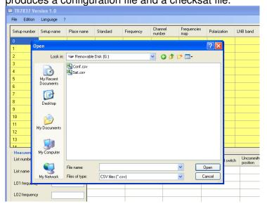
The Conf.csv file is made of the global configuration of the device, the library of setups and the 20 lists of measures.
