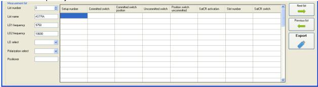
Choose the band selections and the 22 kHz and 13/18 volts polarization, for a universal LNB.
