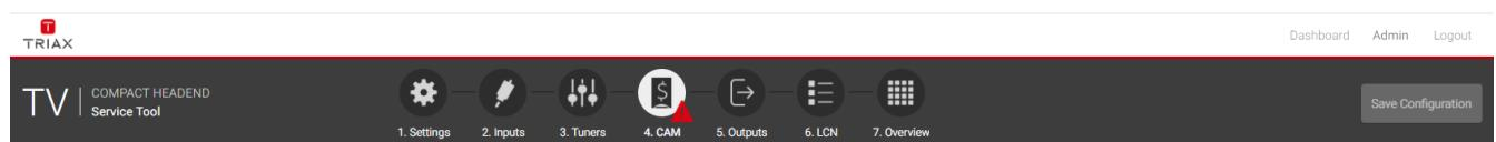
If there is an error in any part of the configuration, the user interface indicates this with a
