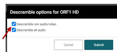
To descramble only selected audio PIDs you have to deselect the Descramble all audio PIDs checkbox. Deselecting the Descramble all audio PIDs checkbox displays a field with a drop-down list below the checkbox.
