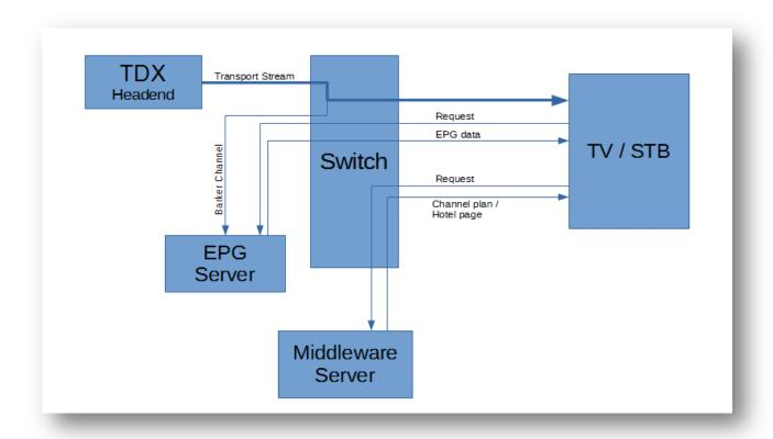
Example setup, based on Macnetix system
